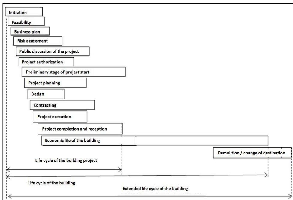
Figure no. 1. Extended life cycle of a building project
